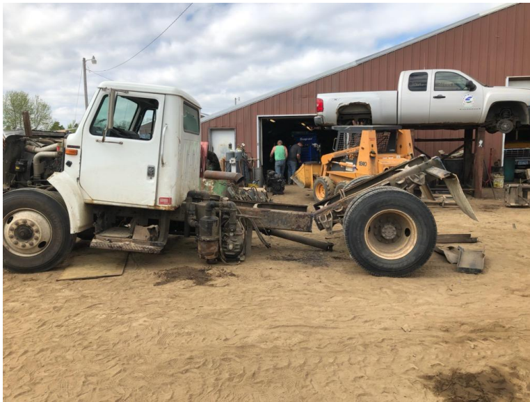
Figure 7. Frame of 1996 International 4700 cut in half.
