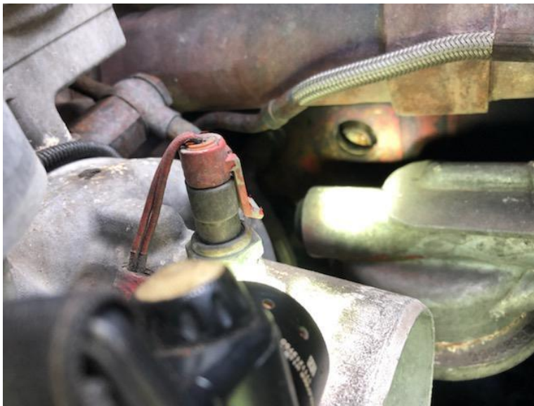
Figure 11. Hole drilled in 2009 Sterling Acterra engine block.
