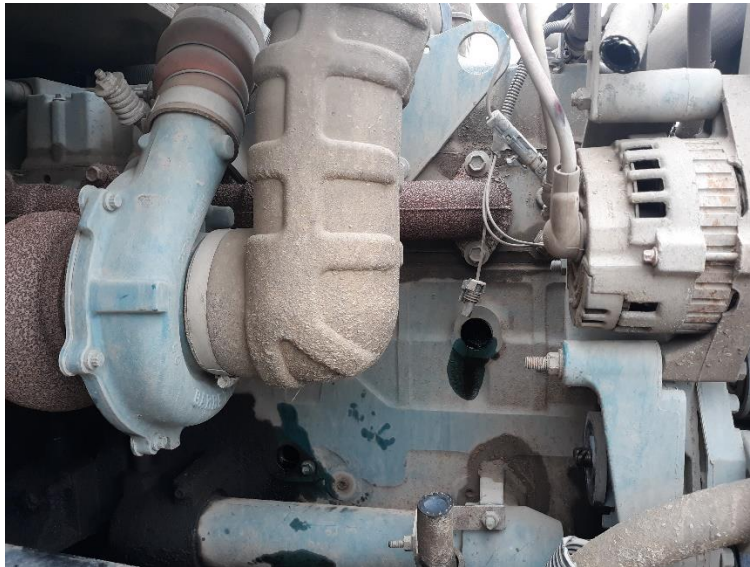
Figure 8. Holes drilled in 1996 International 4700 engine block.
