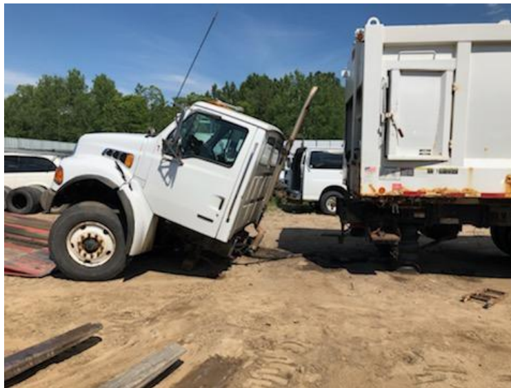
Figure 10. Frame of 2009 Sterling Acterra cut in half.
