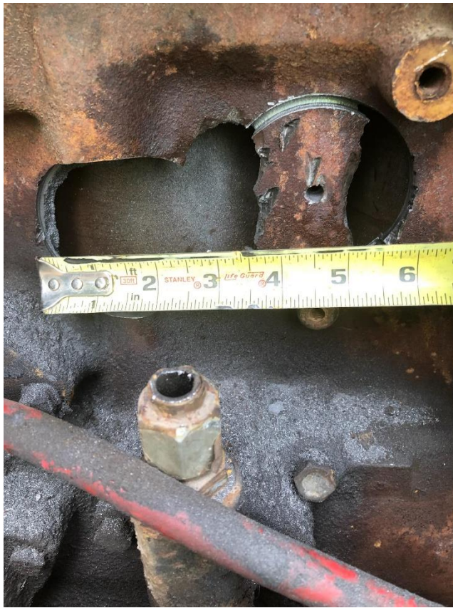
Figure 7. Hole drilled in 1994 Ford engine block.
