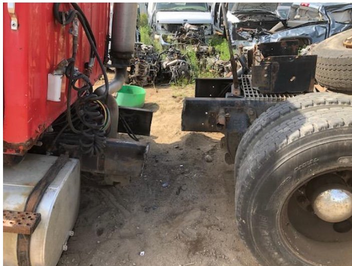
Figure 6. Frame of 1994 Ford cut in half.
