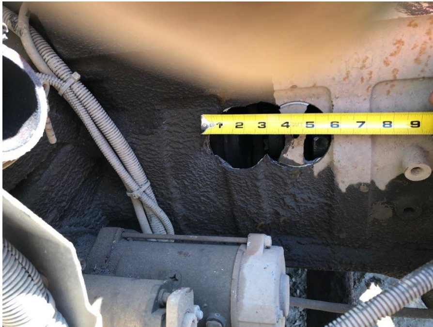
Figure 4. Hole drilled in 1993 Freightliner engine block.
